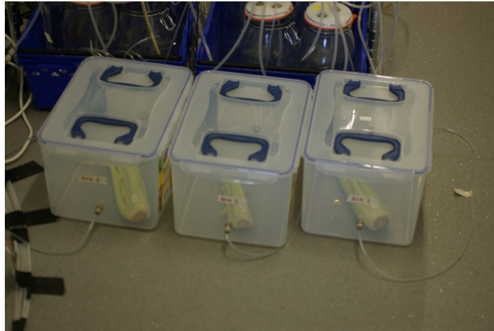
Figure 8 - Air tight plastic boxes connected to the Sable Respirometry System filled with celery samples.
