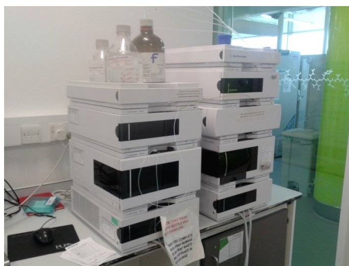
Figure 17 - HPLC-DAD system used to identify and quantify phenolic compounds.
