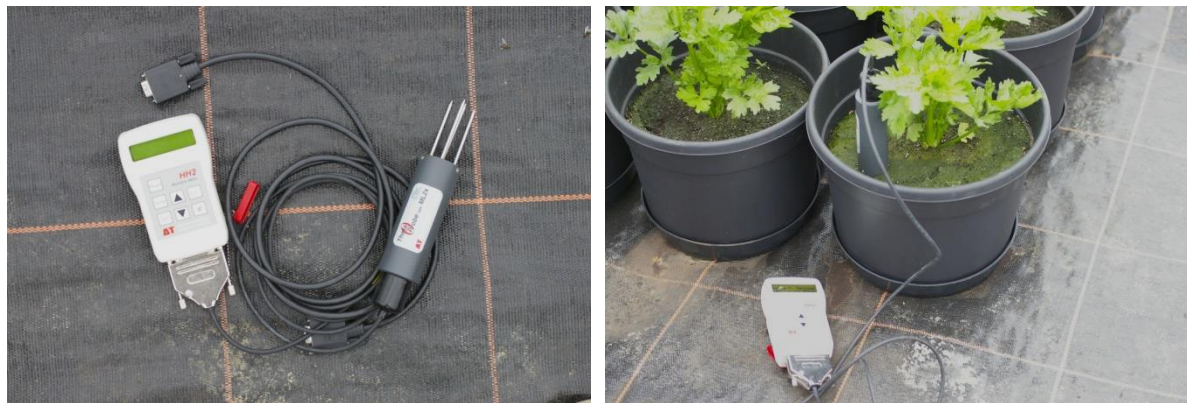
Figure 5 - Thetaprobe meter used to ascertain soil moisture (ThetaKit type ML2x).
