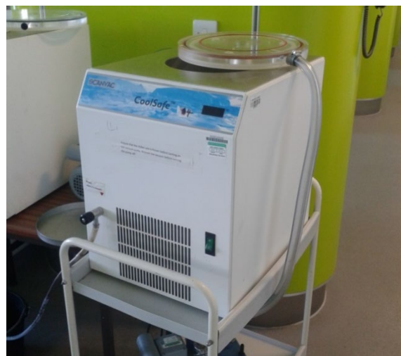
Figure 16 - Freeze-drier used to lyophilize fresh celery samples (Coolsafe 55-9 Scanvac).
