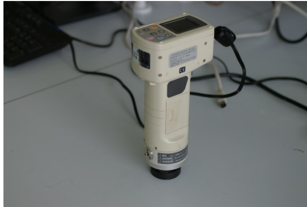
Figure 13 - CR-400 Minolta colorimeter.
